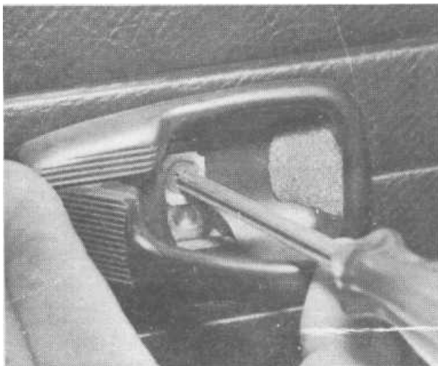
10.1c Remove the escutcheon retaining screw
