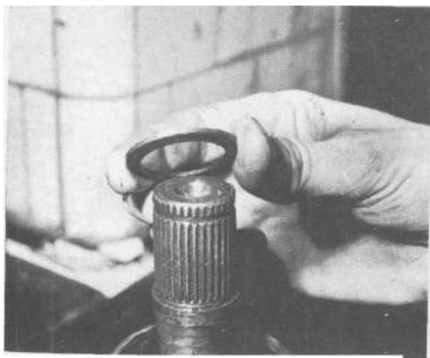
3.5d Discard the concave washer, if one is fitted, behind the joint
