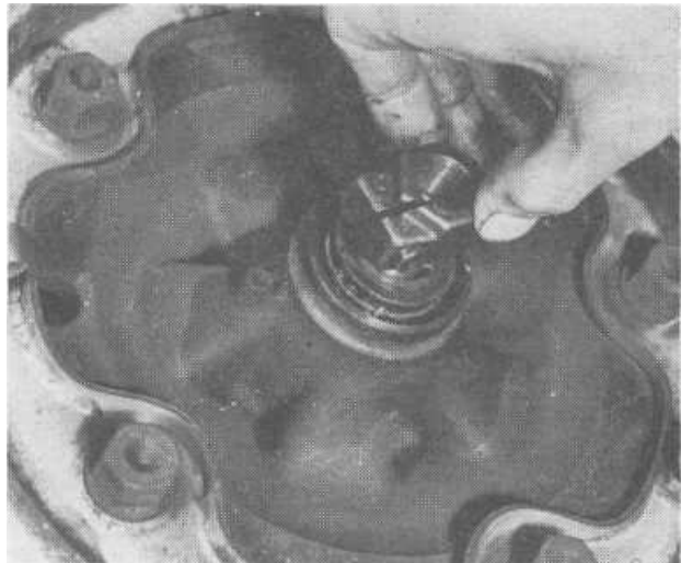
3.7d . . . replace the clamp nut
