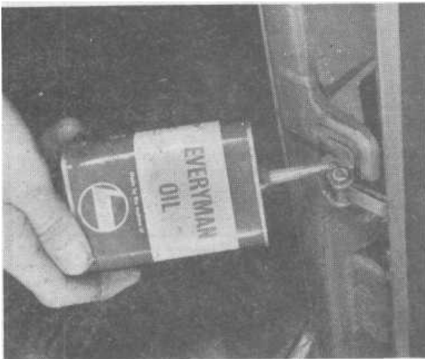
9.4a Check strap lubrication
