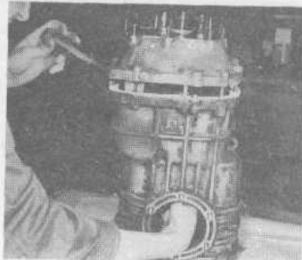
5F.4b It may be necessary to juggle the gear with a screwdriver to get reverse gear onto its shaft
