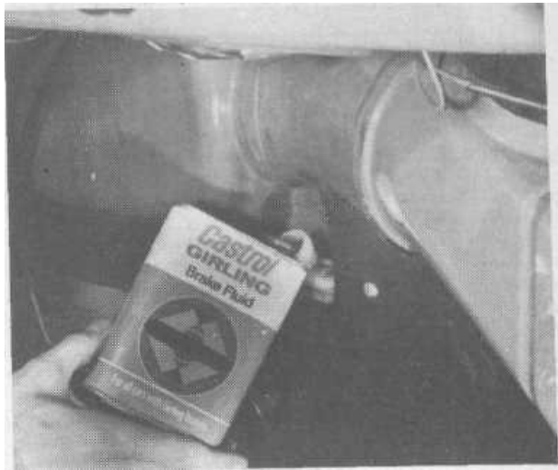
8.6 Filling the master cylinder fluid reservoir
