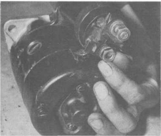
14.2a Undoing the connecting strap terminal nut
