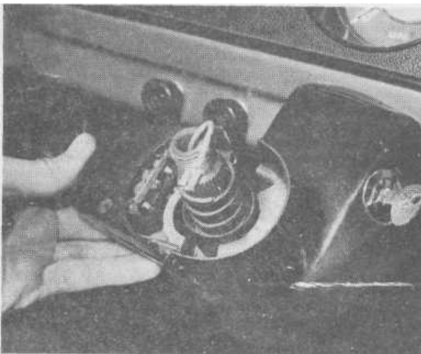
28.1a Undo the screws holding the switch to the column (Note steering wheel has been removed to give a better photo)
